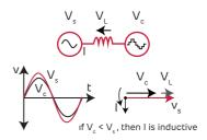
STATCOM in Inductive mode with lagging current output.When VSC voltage smaller in magnitude than system voltage
