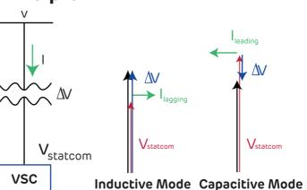
[Inductive mode] If  $V_{statcom}$  is lower than V, the inductive current flows from the AC system to the converter [Capacitive mode] If  $V_{statcom}$  is higher than V, the capacitive current flows the converter to the AC system
