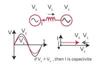
STATCOM in Capative mode with leading current output.When VSC voltage greater in magnitude than system voltage
