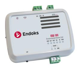
ESU 101 is s cost-effective environmental sensor which is also equipped with Infra Red (IR) controller for split-type Air Conditioners. Thanks to its flexible design, ESU 101 has a learning mode which enables the device to be used with almost all split-type ACs. It has an RS-485 interface supporting Modbus/RTU protocol for SCADA applications.
