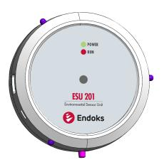
ESU 201 is an advanced environmental sensor which is also equipped with Infra Red (IR) controller for split-type Air Conditioners. Thanks to its flexible design, ESU 201 has a learning mode which enables the device to be used with almost all split-type ACs. In addition, it has low power bluetooth communication protocol, therefore it can be controlled via any device that has bluetooth technology.
