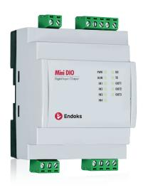
Mini DIO (Digital Input/Output) Module can display on/off or 1/0 data for up to 4 channels. Input channels with high impedance reduce the input current and noise immunity is increased through hysteresis. The device has a anti-jumping filter to prevent contact from jumping. The device also has 32 bit change registers and these registers display the level changes in the input channels.
