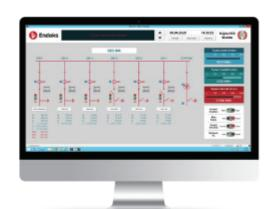
Supervisory control and data acquisition (SCADA) is a system of software and hardware elements that allows industrial organizations to control industrial processes locally or remotely. SCADA monitors, gathers, and processes real-time data directly interacts with devices such as sensors, valves, pumps, motors, and more through human-machine interface (HMI) software and records events into a log file.
